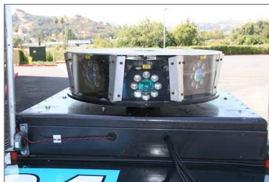
**Figure 10.** Rotating multiple LIDAR system from Team DAD.
