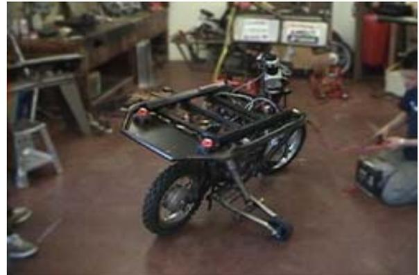
**Figure 18.** Testing of self-righting arms
