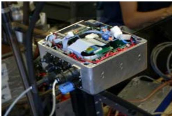
**Figure 8.** Open LDSC with exposed wiring
