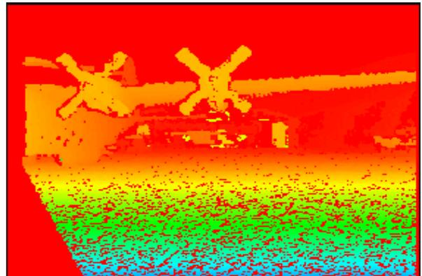
Figure 17. Image of 3D reconstruction with low rejection note invalid background measurements. Color represents distance
