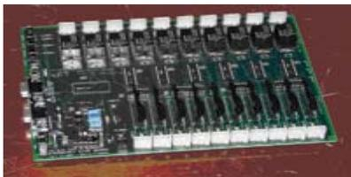
**Figure 11.** E-stop safety receiver interface board
