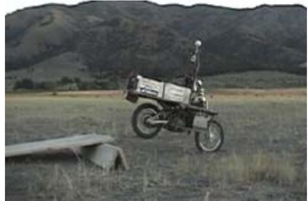
**Figure 6.** Testing of ability to run on bumpy terrain
