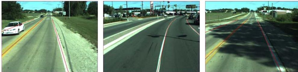
**Figure 4: Examples of lane detection in urban and rural environments**
