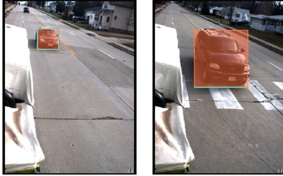
Figure 8: Rear-view System: two examples of vehicle detection.
