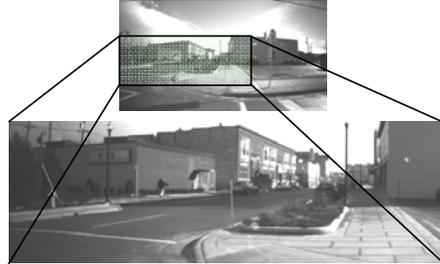
**Figure 7: Lateral System. Top: original low resolution image, a rectangle determines the attentive area; bottom: high resolution image used to detect oncoming traffic**
